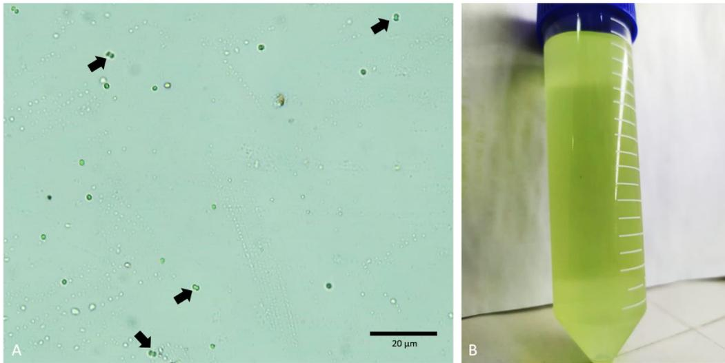
**Figure 2.** (A) Microscopic photographs of *Synechocystis* sp., black arrows show colony of two cells formation and (B) a 50 ml conical flask of 5 days *Synechocystis* sp. culture. The 5 days culture of *Synechocystis* sp. showed green in color. The microscopic photograph showed small size of unicellular *Synechocystis* sp. with some of them formed colonies of two cells
