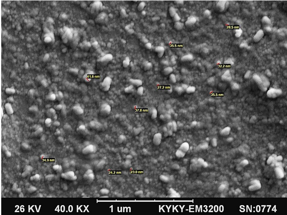
Fig. 2. The SEM image and size range of NPs
