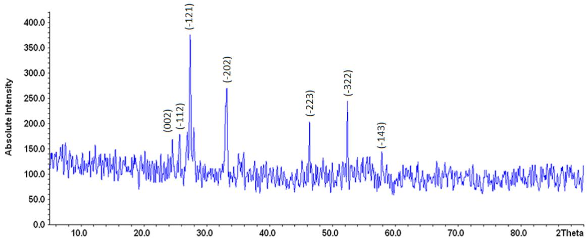
Fig. 3. The X-ray diffraction pattern of BiO NPs
