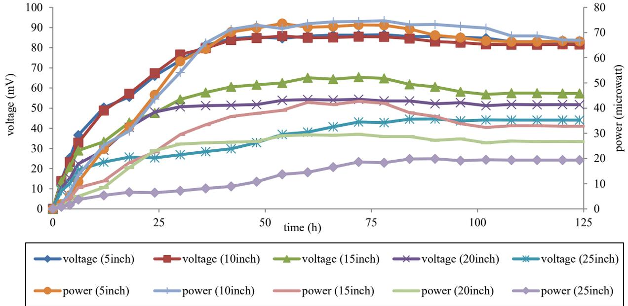
**Figure 4:** Voltage and power generated by MFC using soil of different depth from the palm oil plantation.
