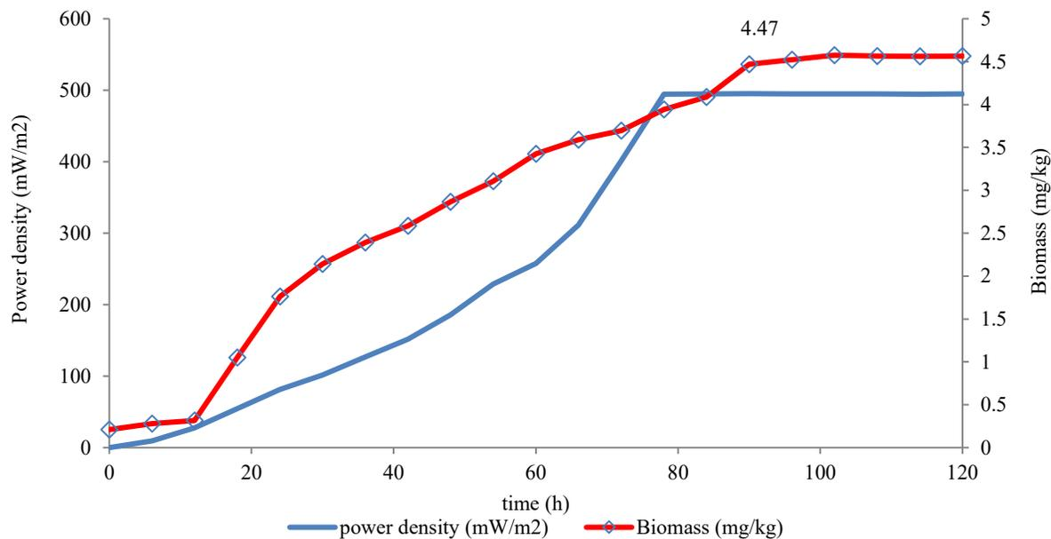
**Figure 8:** Relation between biomass and power generation of optimum ML-MFC and incubation time.
