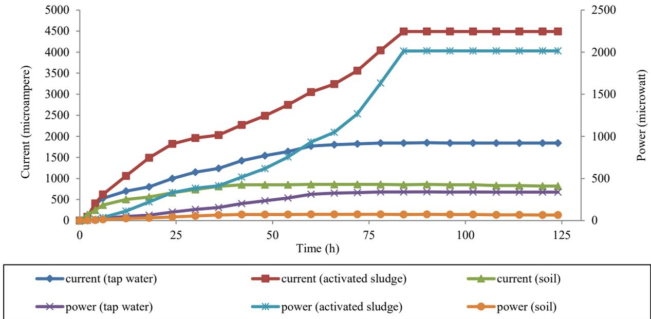
Figure 7: Power and current generated using palm oil plantation soil supplemented with POME activated sludge and tap water.
