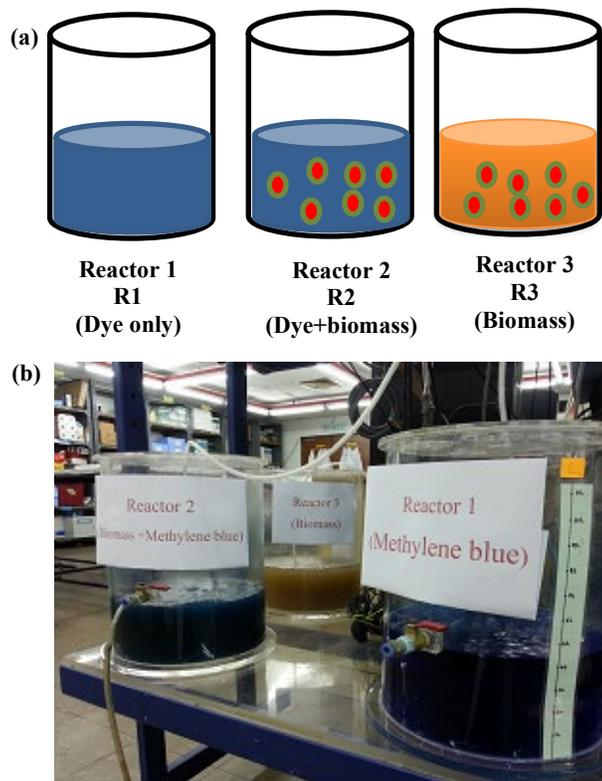
**Figure 1.** (a) Schematic diagram of sequencing batch reactors (SBRs) and (b) laboratory scale of SBRs applied through 14 days of treatment period.
